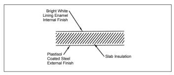
The panel construction as detailed above is a very robust construction giving excellent protection and sound qualities. The construction process involves pressing the panels in a purpose built press, for a period of 24 hours. The external skin is a plastisol coated steel sheet with a 40mm thick zero ODP slab insulation board. The internal skin is a white enamel coated steel sheet, which gives an excellent surface for cleaning and light reflection.
