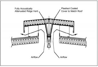
The benefit of the acoustic ridge is that the whole plant room is vented at the highest point, thus ensuring no uneven heat build-up occurs, and if the external temperature rises, the low level louvres allow air to rise within the plant room and escape through the vented ridge.
