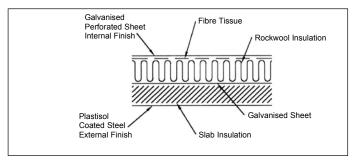
The panel construction as detailed previous is similar to the option B choice but the construction combines the option A panel. This gives a far superior construction and greater sound qualities.
