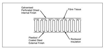
The panel construction as detailed above has the primary function of its excellent sound qualities. It allows sound to be absorbed into the panel thus minimising external noise breakout. The external skin is a plastisol coated steel sheet with 80mm thick rocksil LR insulation. The internal skin is a galvanised perforated steel sheet having a glass fibre tissue membrane affixed thus preventing the migration of the rockwool insulation.
